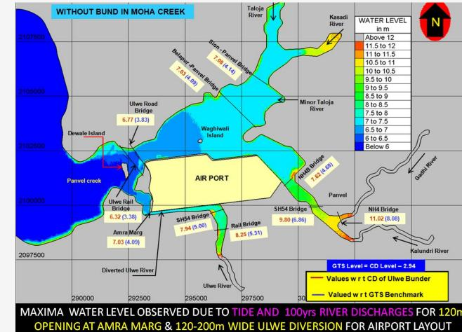
Development level of Airport fixed and Master Drainage Plan for entire surroundings prepared based on CWPRS Studies which considered all climatic conditions including possible changes including tidal variations
