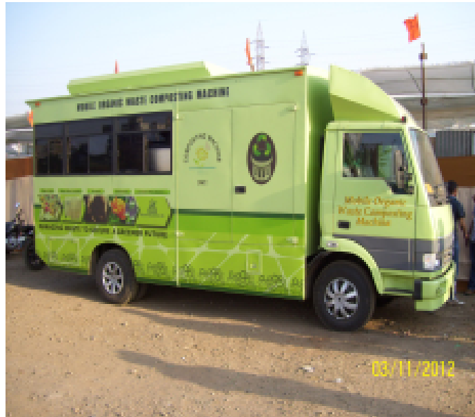
Waste load is 200 kg Power: 4HP 200kw Capacity: 200 kg/day
